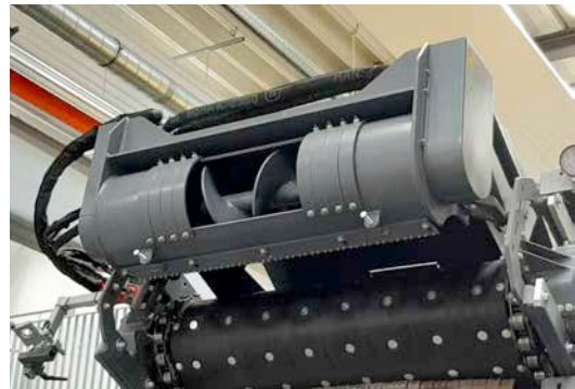
FLEXMIX mixing unit can be folded up hydraulically.
