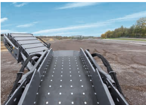
Flexible in use – the optionally available swivel belt with 6.5 m (OC 650) for BMF 2500 S.
